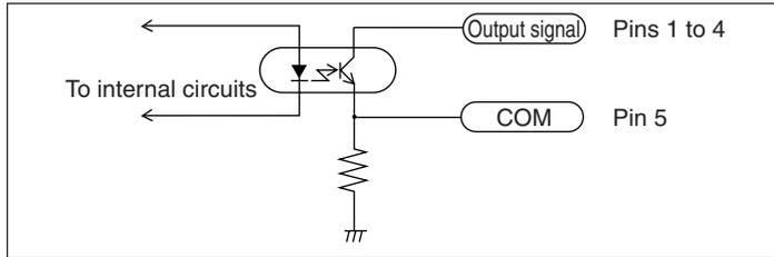
When using the general-purpose output as the reference point output, time until the output signal changes to High is 200 ms after going past the reference point.
