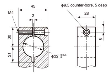
Tightening torque: 6 N·m Hex. socket head bolt M5 is used.
