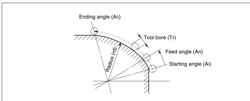
Reducing the feed angle produces a cleaner finish.
