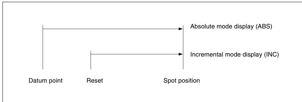
The conversion between the absolute mode (ABS) and incremental mode (INC) can be made by pressing:
