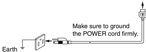
If your model contains both a 100-120 V power cord and 200-240 V power cord, use the proper power cord for the operating voltage.
