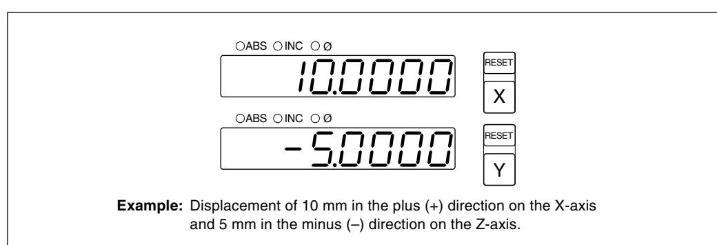
**Example:** Displacement of 10 mm in the plus (+) direction on the X-axis and 5 mm in the minus (-) direction on the Z-axis.
