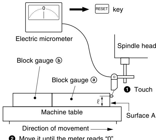
**3** Next, move the table away from the probe and remove the block gauge ④, move the machine table again, touch the surface C of the block gauge ⑤ with the probe of the electric micrometer or dial gauge, and move the machine table until the meter reads "0". The difference between the length L of the block gauge ④ and the displayed value on the counter unit is the linear error to be compensated.
