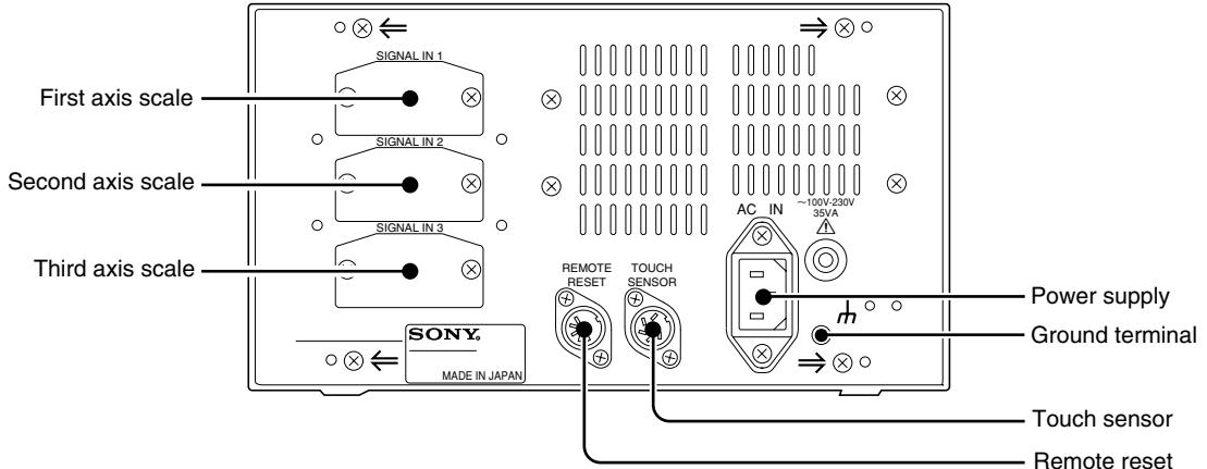
**⚠** For safety sake, be sure to connect the supplied power cord in between ground terminal of unit and ground.
